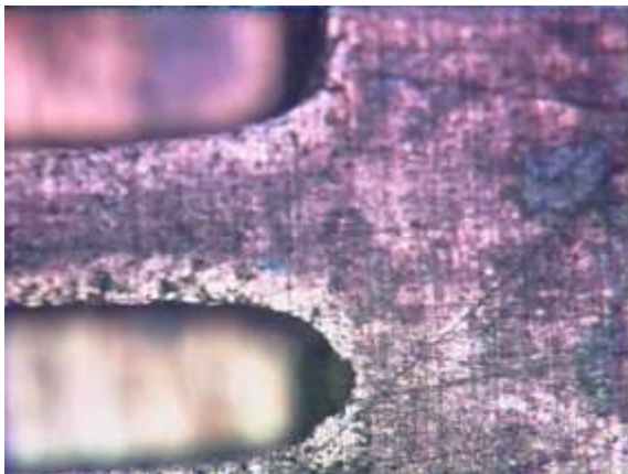
Figure 8. Internal view of turbulent region of a copper MCCP showing no change in the surface of the unplated copper channels after 2,000 hours of operation in optimum DI water.
