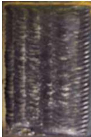
Figure 9 - HPDDL wire feed clad – performed in the vertical position using standard 0.8 mm diameter wire
