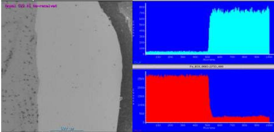
Figure 6: A SEM line trace of a NiCrMo clad produced at 0.45 m/min, 4 kW.
