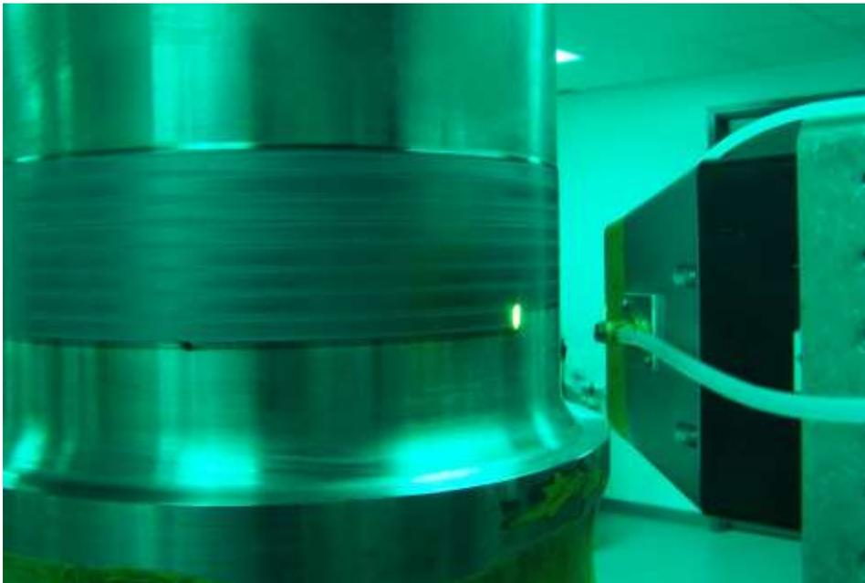
Figure 2 – HPPDL surface hardening bearing surface on large axel
