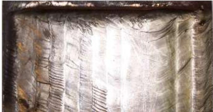
Figure 8 –HPDDL wire feed clad – performed in the horizontal position using standard 0.8 mm diameter wire.
