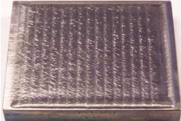
Figure 4 – HPDDL clad mild steel substrate – [200 X 200 X 25 mm] 1.5 mm thick nickel chrome clad
