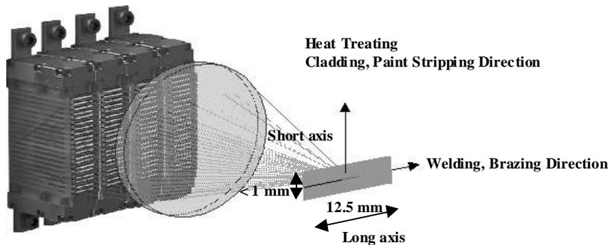
Figure 1 – HPDDL Standard Line focus configuration
