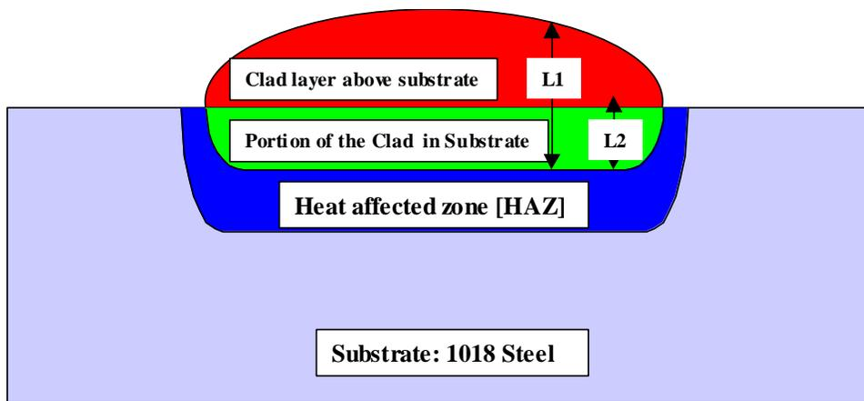
Figure 5: Standard visual measurement of dilution was performed through the equation  $L2/L1$ .
