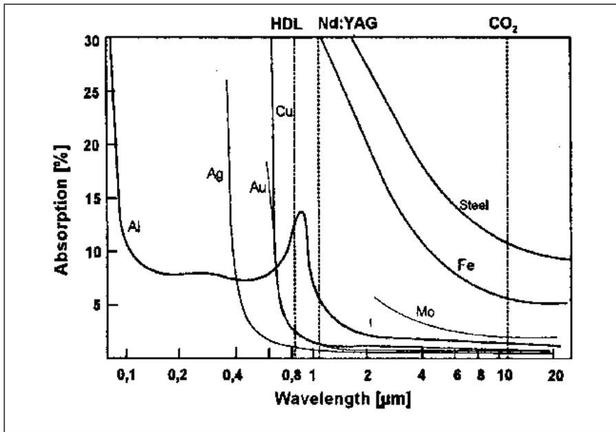
Figure 3 - Absorption vs. Wavelength for typical metals<sup>4,5</sup>
