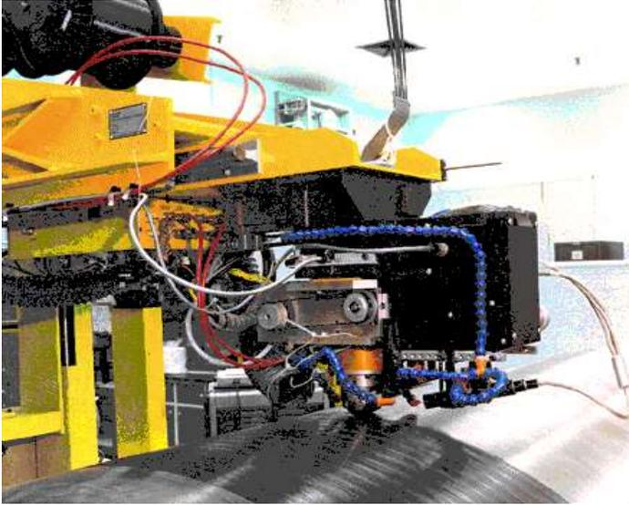
Figure 3 – McDonnell Douglas Aircraft CO<sub>2</sub> laser assisted fiber placement machine circa-1995.
