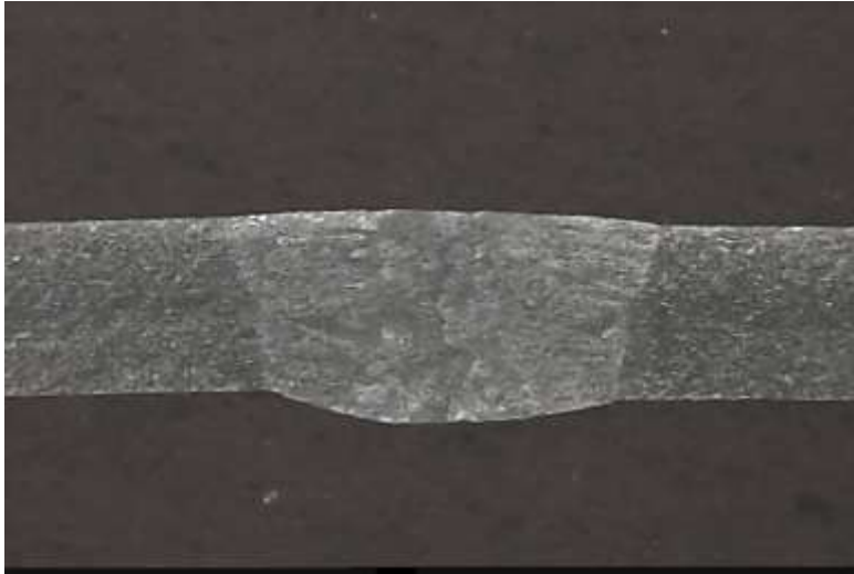
Figure 12: The fusion zone and heat affected zone of a 5754 aluminum laser weld.
