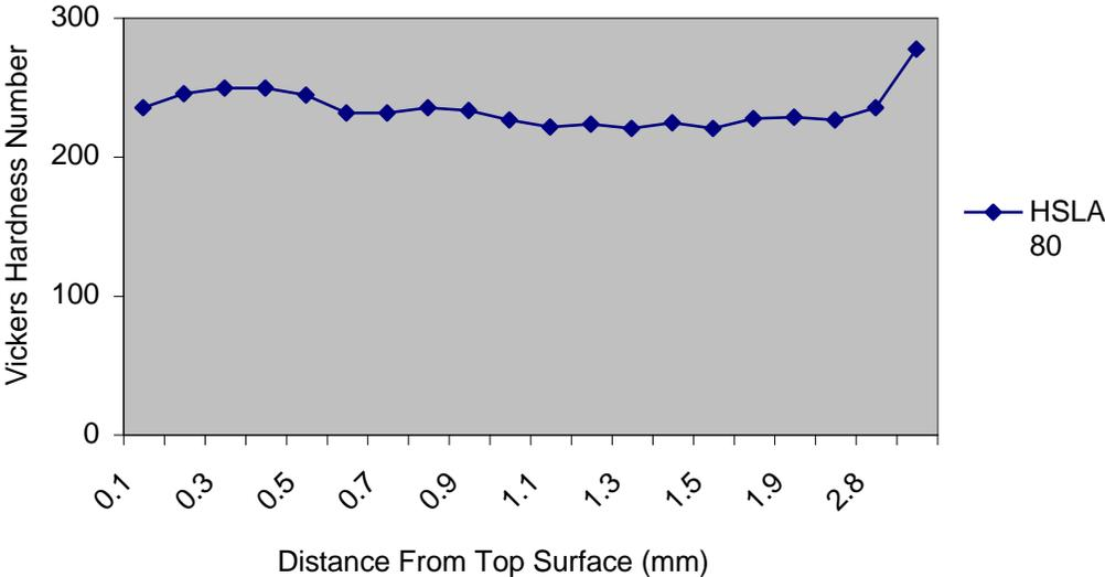
Figure 13: Vickers Hardness Number Versus Distance From Top Surface in HSLA 80 Laser Assisted Forming
