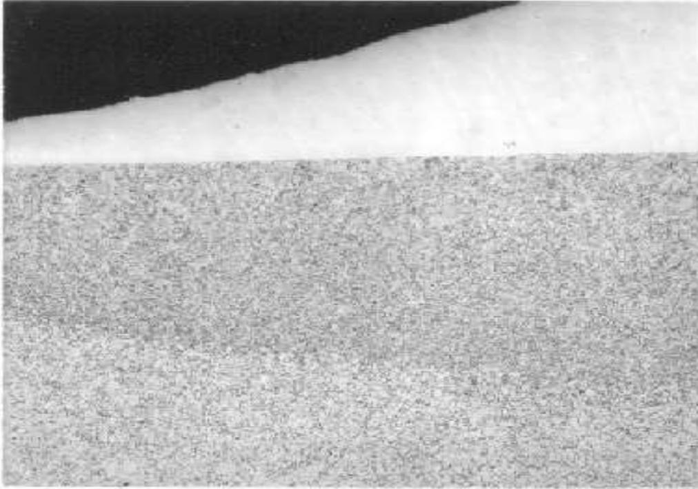
Figure 9: Inconel 625 clad taken at a magnification of 50X.
