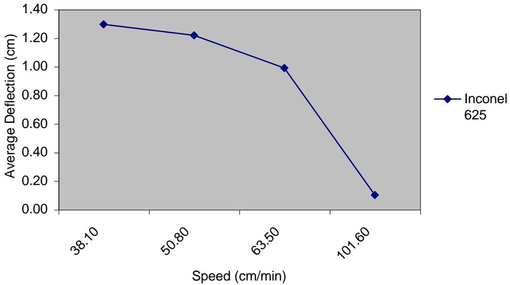
Figure 12: Average Deflection Versus speed in Inconel™625 Laser Assisted Forming
