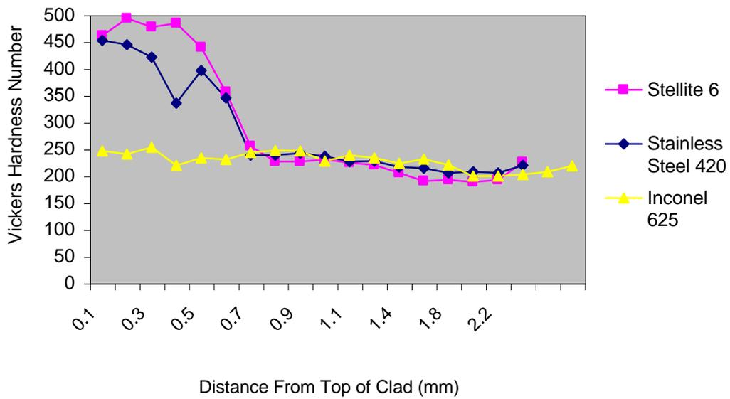
Figure 10: Vickers Hardness Number Versus Distance From Top of Clad
