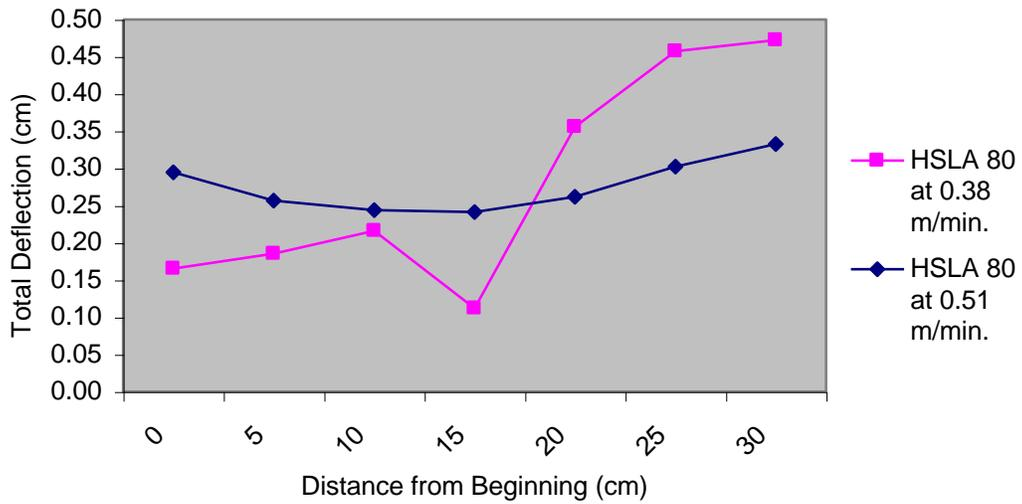
Figure 11: Comparison of Deflection Versus Distance From Beginning in HSLA 80 Steel Laser Assisted Forming
