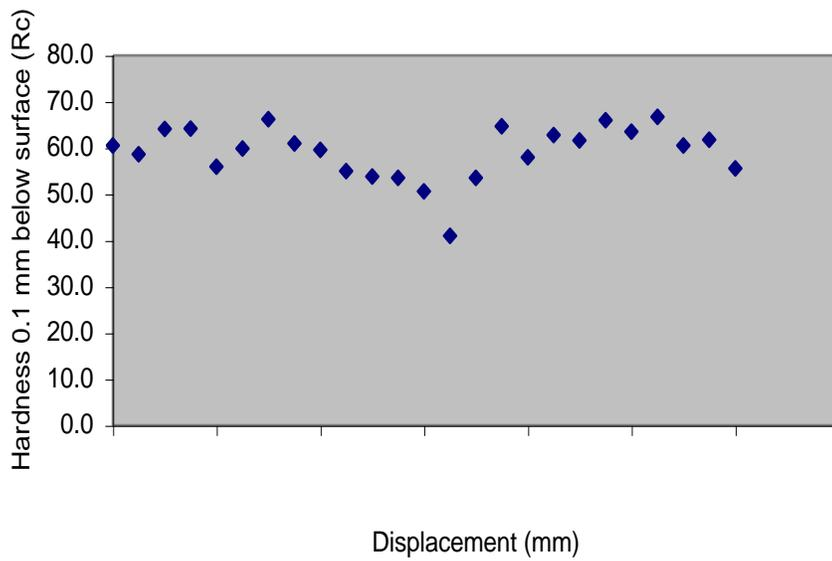
Figure 4: Superhardening has occurred in this sample as seen in the high hardness values obtained 0.1 mm below the surface.
