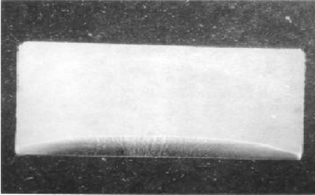
Figure 7: This photograph demonstrates the surface hardening in a 4140 steel. This picture was taken at a magnification of 6X.
