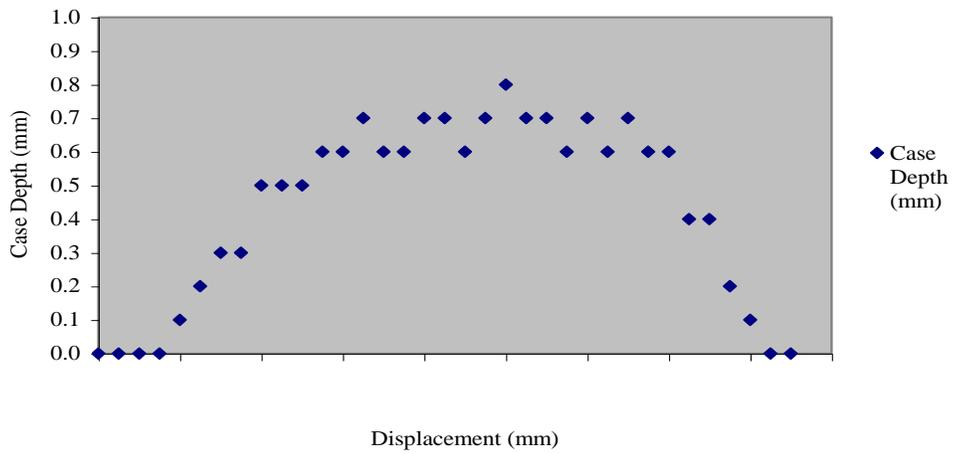
Figure 3: The hardened zone produced from a single pass, laser beam surface treatment. The beam profile is typically Gaussian as shown in the above graph.
