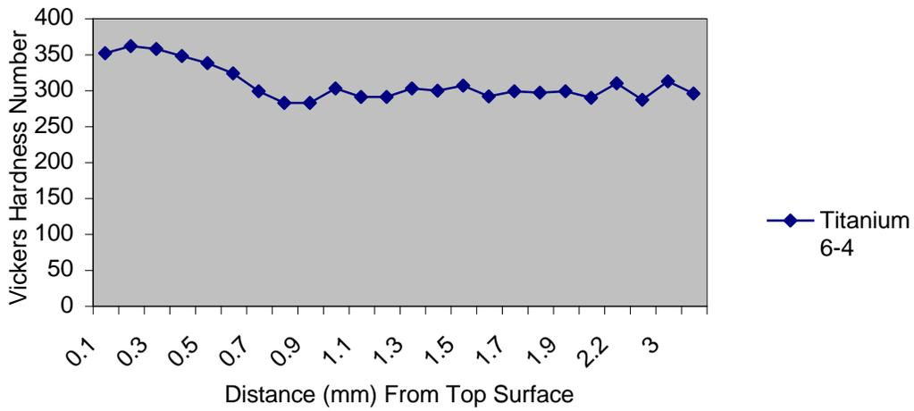
Figure 8: Vickers Hardness Number Versus Distance From Top Surface in Titanium 6-4
