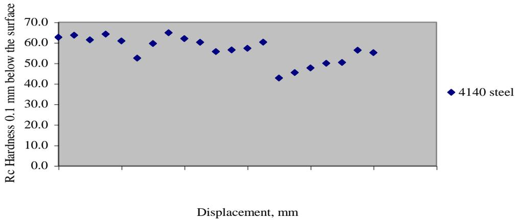
Figure 5 : This figure demonstrates the effect of backtempering on hardness of a sample. The second beam was moved over 13mm after the first pass. Note, that the superhardened zone is immediately followed by the back tempered zone.
