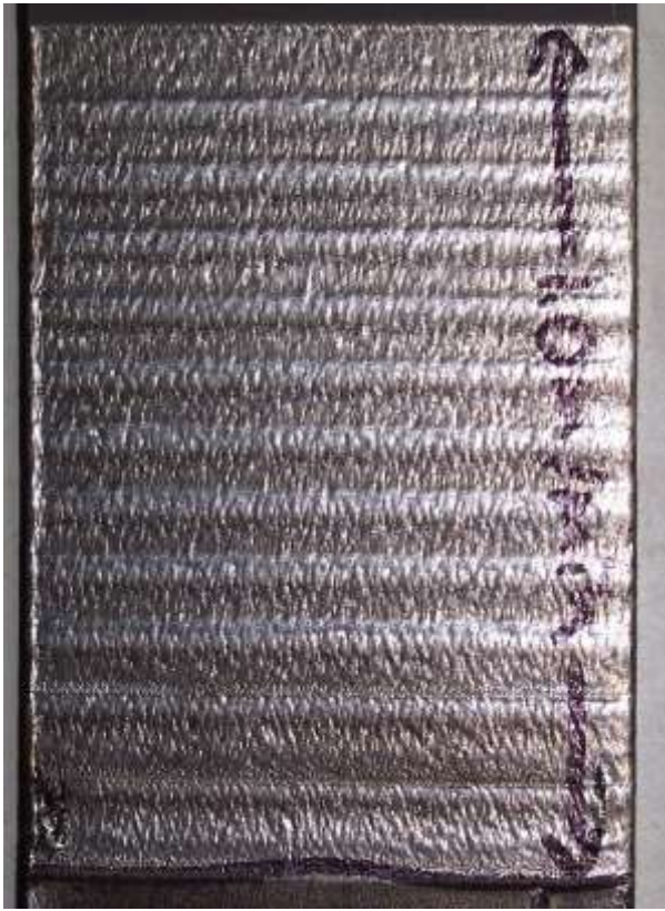
Figure 5 – Resulting LSI surface from ISL-4000L HPDDL – Process speed 1.0 m/min @ 4000W
