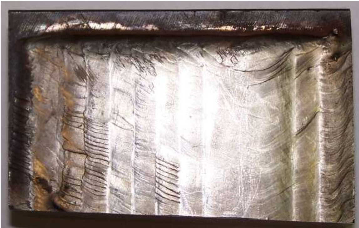
Figure 10 - Result of HPDDL wire feed cladding. 4 layers of overlapping Inconel 625 wire 0.2 m/min @ 4000 w
