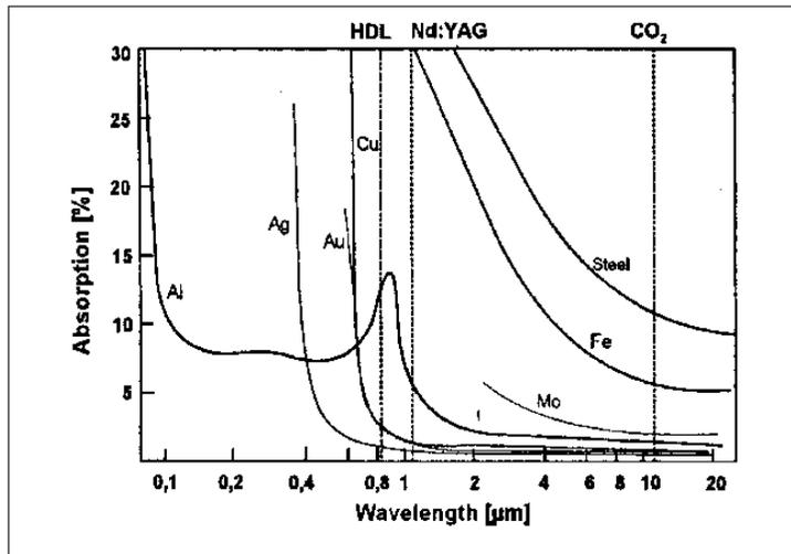
Figure 5 - Absorption vs. Wavelength for typical metals
