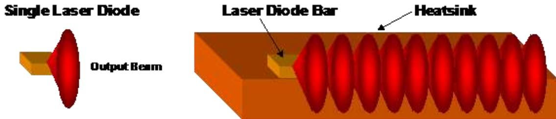
**Figure 1 - Configurations of HPLLD Bar**
