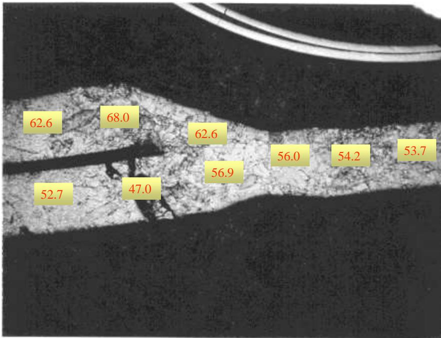
**Figure 10: Micrograph of galvanized steel lap weld, 18.5 X magnification, 2% Nital etch.**
