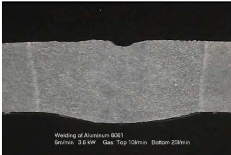
**Figure 14: Micrograph of Aluminum 6061 weld at 6M/min.**
