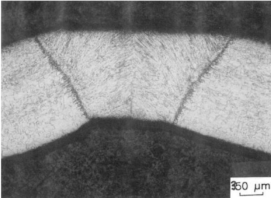
**Figure 7: 304 Stainless Steel Tube Weld**
