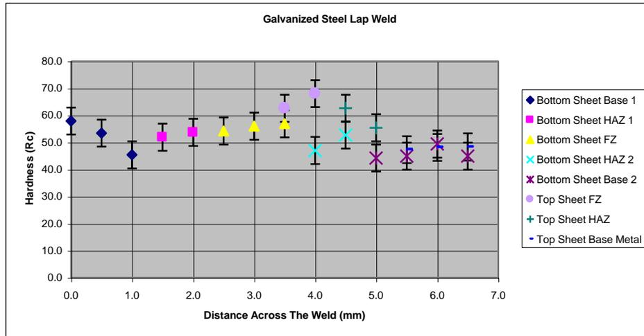
**Figure 11: Average hardness plotted against distance across the weld for galvanized steel lap weld.**
